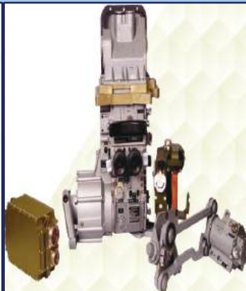
Commander's Sighting and Vision System PNK-4S
